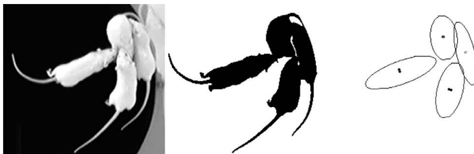
Fig. 1. Original image (left), segmented image using background subtraction (center) and the results of the k -means clustering procedure with results shown in ellipses (right).
